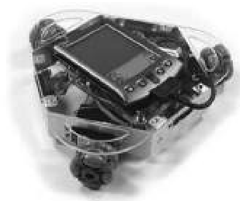
Fig.3.26 Robot with three omnidirectional wheels
