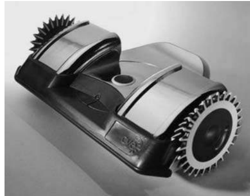
Fig.3.9 Cye, a commercial two-wheel differential-drive robot
