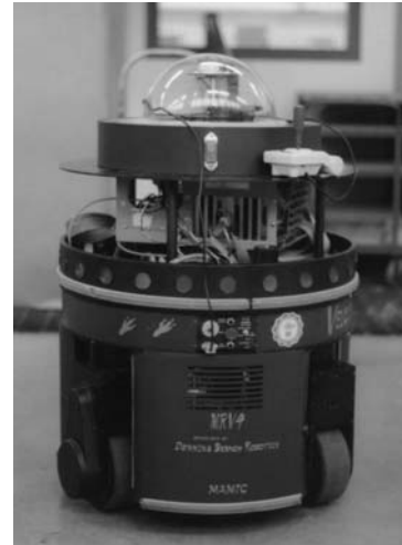
Fig.3.17 MRV4 robot with synchro drive mechanism
